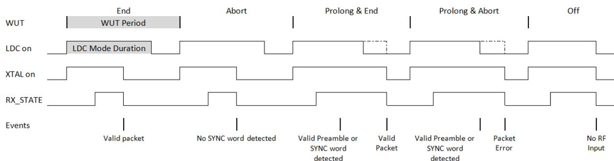
**Figure 14. Low Duty Cycle Mode for RX**
