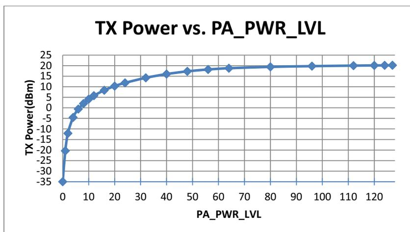
Figure 7. +20 dBm TX Power vs. PA\_PWR\_LVL
