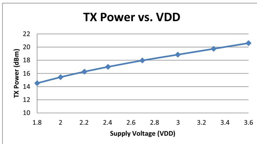
Figure 8. +20 dBm TX Power vs. VDD
