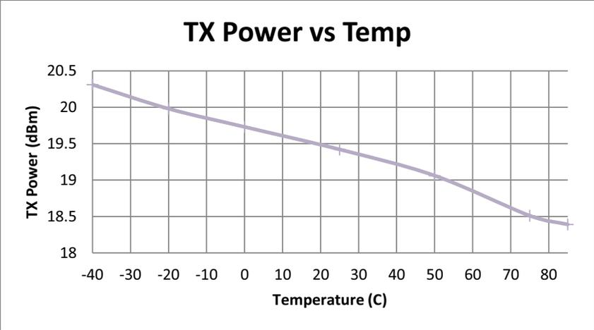
Figure 9. +20 dBm TX Power vs. Temp
